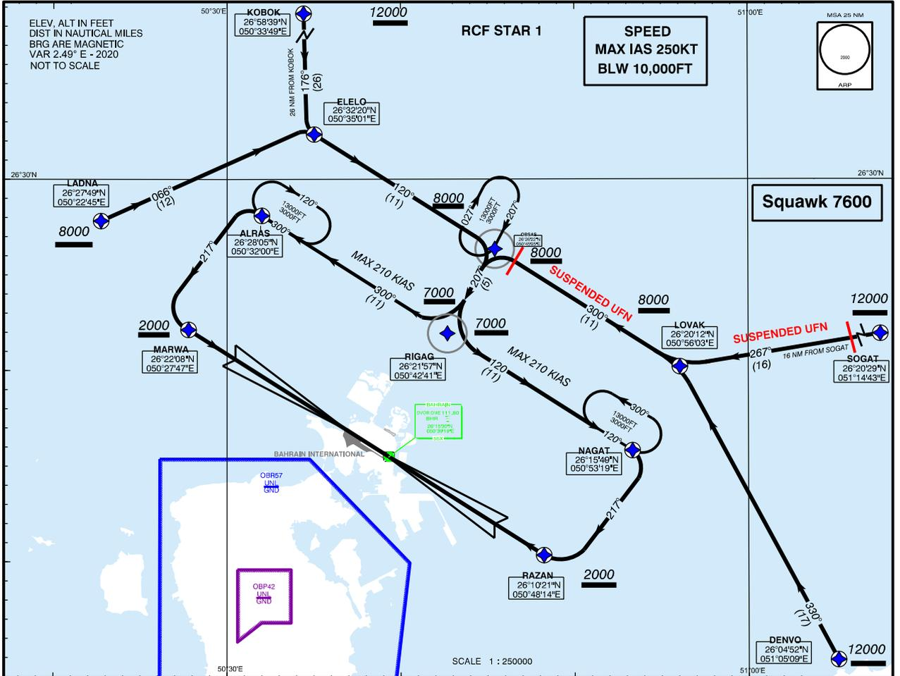
**RADIO COMMUNICATION FAILURES STAR (RNAV1)**
